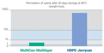
Used for oxygen-sensitive and/or liquids tending to permeation
